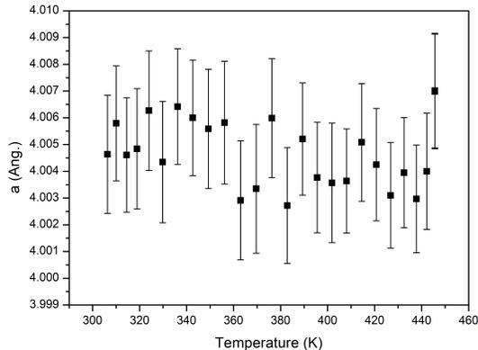
FIG. 9. The  $a$  unit cell parameter of LaFeSi as a function of temperature, during cooling.
