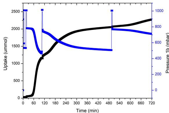
FIG. 7. The uptake of deuterium plotted with the deuterium injection curves
