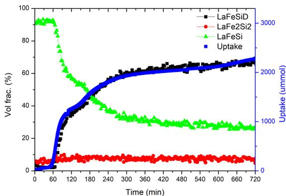
FIG. 5. Volume fraction of phases as determined by NPD plotted with the calculated deuterium uptake.
