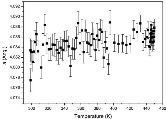
FIG. 1. The  $a$  unit cell parameter of LaFeSi as a function of temperature, during heating.
