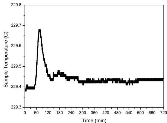
FIG. 8. The temperature of the sample as a function of time. A peak is seen at the start of the reaction indicating an exothermic behaviour.
