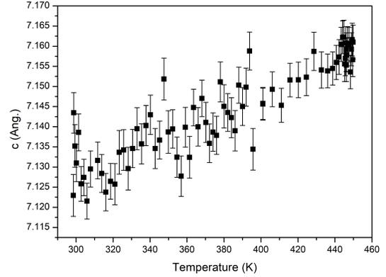
FIG. 2. The  $c$  unit cell parameter of LaFeSi as a function of temperature, during heating.
