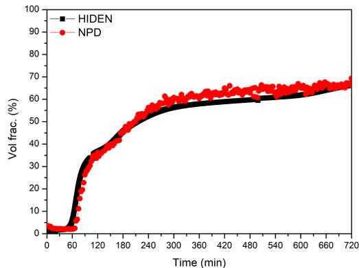
FIG. 6. Volume fraction of LaFeSiD as determined by NPD and from the Deuterium uptake.
