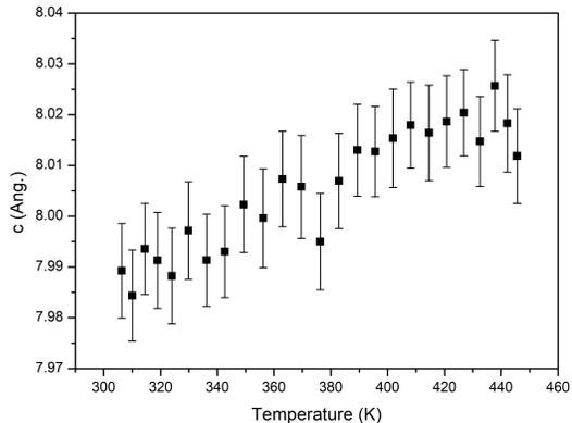
FIG. 10. The  $c$  unit cell parameter of LaFeSi as a function of temperature, during cooling.
