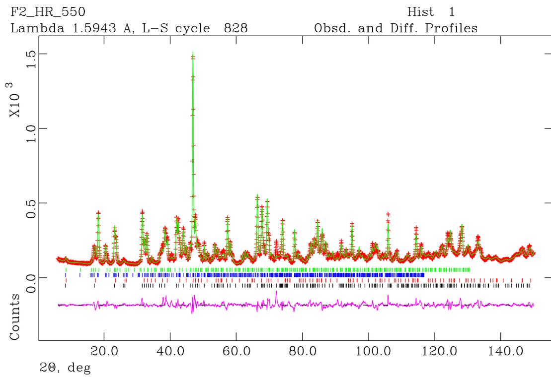
Figure 2. NPD fitted profiles for  $\text{La}_2\text{BaFe}_2\text{O}_6\text{F}_2$ .
