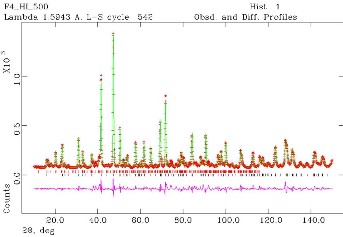
Figure 1. NPD fitted profiles for  $\text{La}_2\text{BaFe}_2\text{O}_5\text{F}_4$ .
