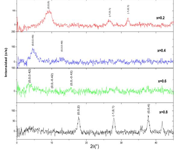
FIG. 2. Principal magnetic peaks of  $\text{Dy}(\text{Co}_x\text{Ni}_{1-x})_2\text{B}_2\text{C}$  as determined from the neutron diffractograms measured at  $T=1.5$  K.
