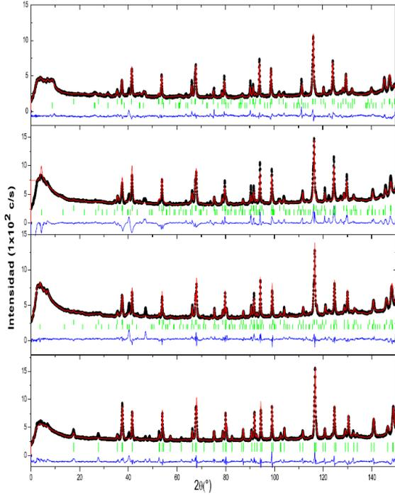
FIG. 1. Neutron diffractograms of  $\text{Dy}(\text{Co}_x\text{Ni}_{1-x})_2\text{B}_2\text{C}$  (from top to bottom  $x=0.2, 0.4, 0.6$  and  $0.8$ ) measured at  $T=1.5$  K. The solid line represent the Rietveld refinements parameters as given in Table 1.
