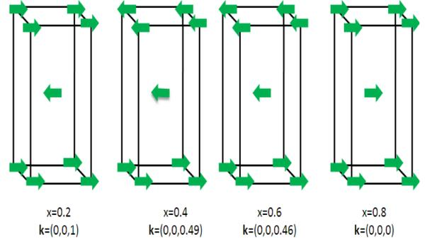
FIG. 3. Magnetic structure of  $\text{Dy}(\text{Co}_x\text{Ni}_{1-x})_2\text{B}_2\text{C}$  as determined from neutron diffraction analysis.
