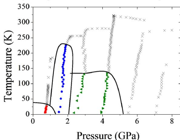
**Figure 1** Points of the Pressure Temperature for which a powder pattern was obtained on D20. Red dots correspond to the helimagnetic phase. Blue and Green dots correspond to the new observed magnetic phases
