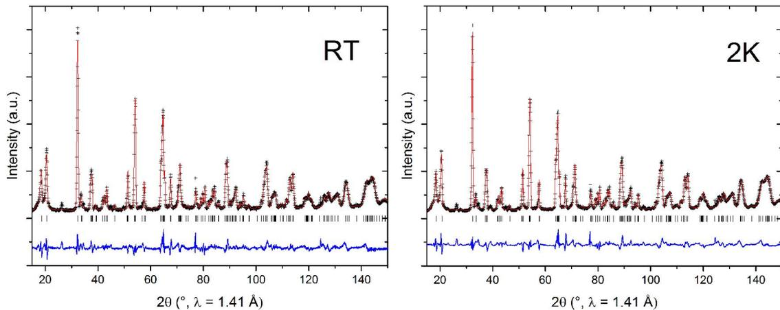
Figure 2: Neutron diffraction pattern of  $\text{Li}_3\text{FeN}_2$  recorded at room temperature and 2K.
