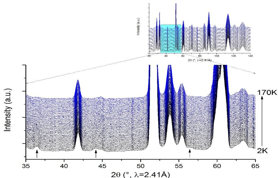
Figure 3: Neutron diffraction patterns recorded from 2K to 170K.
