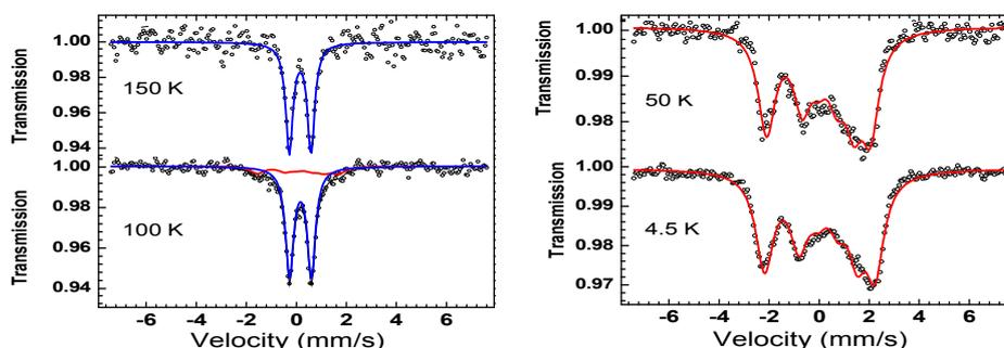
Figure 1: Mössbauer spectra of  $\text{Li}_3\text{FeN}_2$  recorded at 150, 100, 50 and 4.5K respectively.
