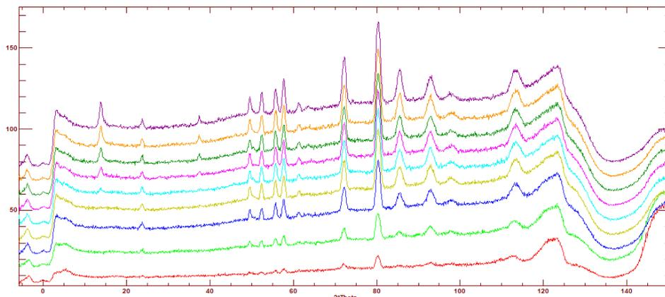
**Fig. 2** Diffraction patterns taken while warming the sample at 7 GPa. Topmost pattern is at 80 K, bottom is at room temperature. A subset of curves is shown and they are offset for clarity.
