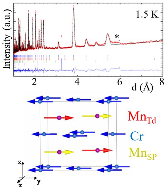
Fig. 1. Magnetic structure of the CaMnCrSbO<sub>6</sub> DDPv as refined from 1.5 K NPD data.
