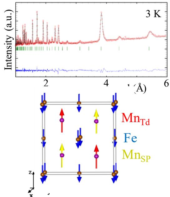
Fig. 2. Magnetic structure of the CaMnFeSbO<sub>6</sub> DDPv as refined from 3 K NPD data.
