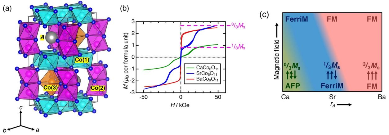
**Figure 1.** (a) Crystal structure of  $ACo_6O_{11}$  ( $A = Ca, Sr, Ba$ ). (b) Isothermal magnetization curves at 1.8 K for polycrystalline  $ACo_6O_{11}$  ( $A = Ca, Sr, Ba$ ). (c) Magnetic phase diagram of  $ACo_6O_{11}$  ( $A = Ca, Sr, Ba$ ).
