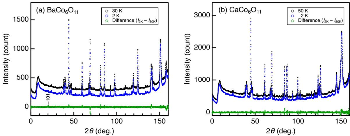
**Figure 2.** (a) NPD patterns of  $BaCo_6O_{11}$  collected at 30 K (black) and 2 K (blue) in zero field using D2B diffractometer, and their difference (green). (b) NPD patterns of  $CaCo_6O_{11}$  collected at 50 K (black) and 2 K (blue) in zero field using D2B diffractometer, and their difference (green).
