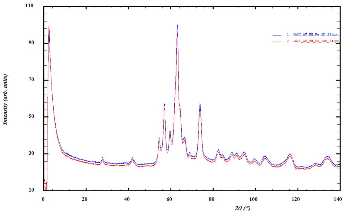
Figure 2: NPD patterns of sample JACC\_AW\_BM\_Fe upon heating (2K in blue and 10K in red)
