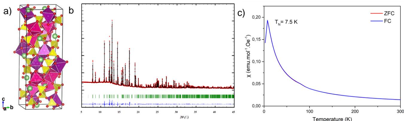
Figure 1: (a) Structural model proposed by Isasi *et al.*<sup>5</sup> for  $\text{Li}_2\text{Mn}_2(\text{SO}_4)_3$ . (b) Rietveld refinement of this structural model against the Synchrotron XRD pattern of a sample  $\text{Li}_2\text{Mn}_2(\text{SO}_4)_3$ . (c) Temperature dependent magnetic susceptibility of a sample of  $\text{Li}_2\text{Mn}_2(\text{SO}_4)_3$  indicating long-range ordering at 7.5K.
