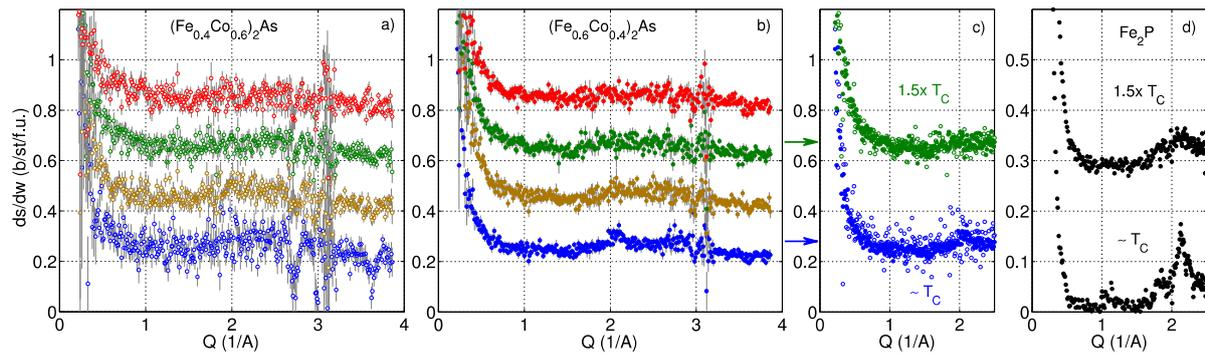
**Figure 3.:** Magnetic scattering cross section ( $ds/dw$ ) as a function of wave vector transfer  $Q$  for a)  $(\text{Fe}_{0.4}\text{Co}_{0.6})_2\text{As}$  measured at 270, 275, 390, and 525 K (bottom up) and b)  $(\text{Fe}_{0.6}\text{Co}_{0.4})_2\text{As}$  at 325, 425, 480, and 525 K (bottom up). C + d) shows comparison of the raw data for  $(\text{Fe}_{1-x}\text{Co}_x)_2\text{As}$  and  $\text{Fe}_2\text{P}$  at  $\sim T_C$  and  $1.5x T_C$ .
