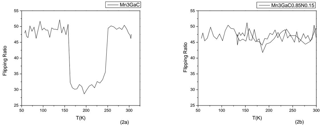
Fig2. Temperature dependence of value of flipping ratio for (a)  $\text{Mn}_3\text{GaC}$  and (b)  $\text{Mn}_3\text{GaC}_{0.85}\text{N}_{0.15}$ .
