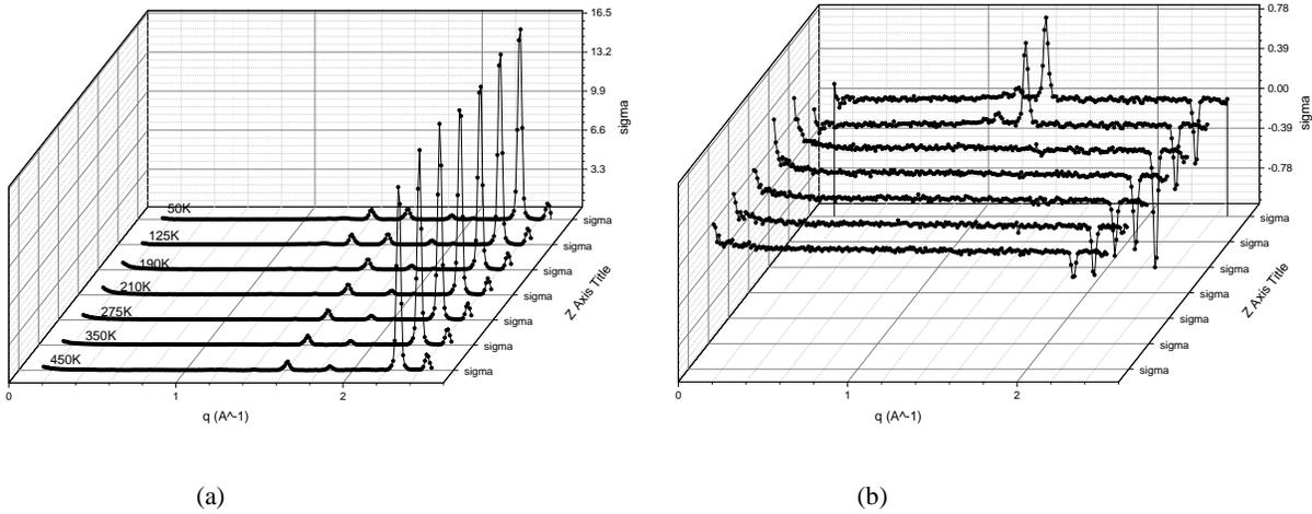
Fig. 4 the total and magnetic scattering cross sections for  $Mn_3GaCN$  (a) total (b) magnetic
