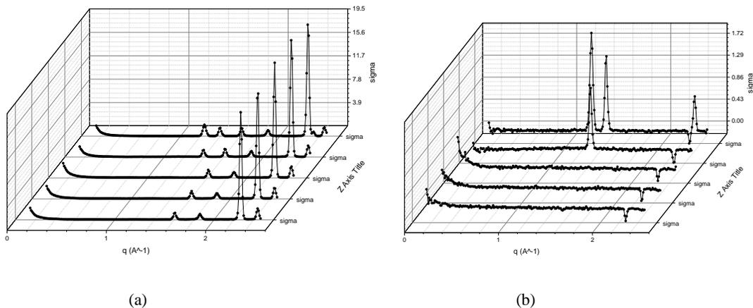
Fig 3 the total and magnetic scattering cross sections for  $\text{Mn}_3\text{GaC}$  (a) total (b) magnetic
