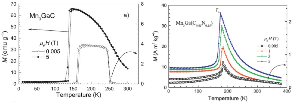
Fig1: Temperature dependence of the magnetization measurements. (a) under 5 mT (right scale) and 5T (left scale) for  $\text{Mn}_3\text{GaC}$ . (b) under 5 mT (right scale) and 1, 3, 5 T (left scale) for  $\text{Mn}_3\text{GaC}_{0.85}\text{N}_{0.15}$
