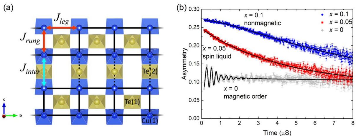
Figure 1. (a) The spin ladder structure of  $\text{Ba}_2\text{CuTe}_{1-x}\text{W}_x\text{O}_6$ . The  $\text{W}^{6+}$  cations are substituted onto the corner-sharing  $\text{Te}(1)$  site allowing the direct tuning of interactions in the ladder. (b) Muon spin rotation and relaxation measurements on  $x = 0.05$  and  $x = 0.1$ , which reveal the lack of magnetic ordering.
