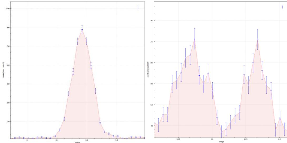
**Fig. 1.** Integration of the collected  $\omega$ -scans around the (1 -1 2) nuclear and (0.5 0 1.5) magnetic reflections. In order to reduce the background contribution the integration was done using a region of interest around the observed reflection.
