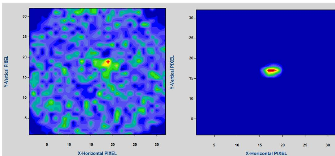
**Fig. 2.** 2D plots at the center of the  $\omega$ -scan for the (0.00 -0.48 1.56) magnetic reflection (left), and (1 -1 2) allowed nuclear reflection at 2 K.
