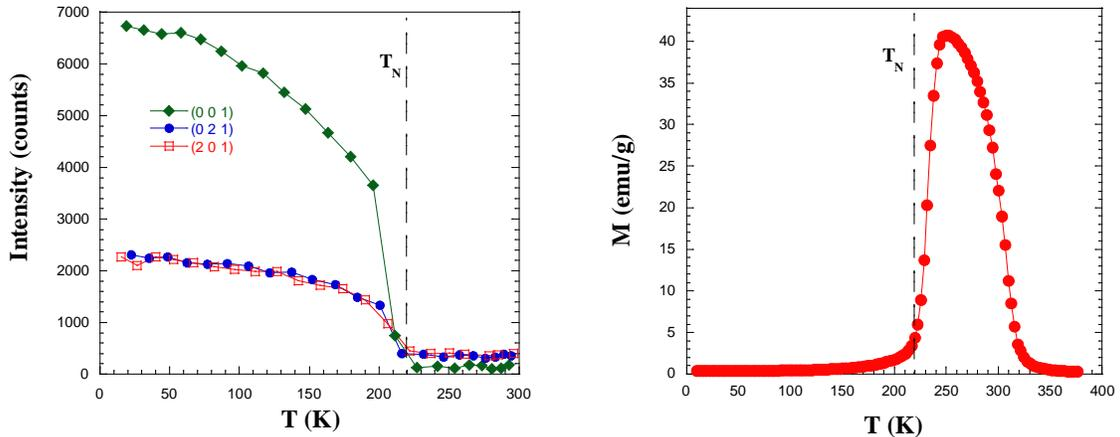
**Fig. 1.** Temperature dependence for the intensity of selected magnetic reflections (left). Magnetization as a function of the temperature for PBMO crystal (right).
