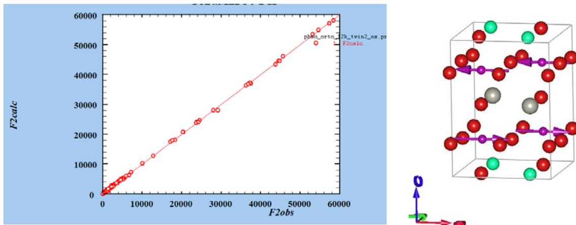
**Fig. 2.** Left: Calculated versus observed values of the squared intensities for refined single crystal neutron diffraction data collected at 12 K for PBMO following the model  $A_xG_yF_z$ . Right: Corresponding magnetic structure.
