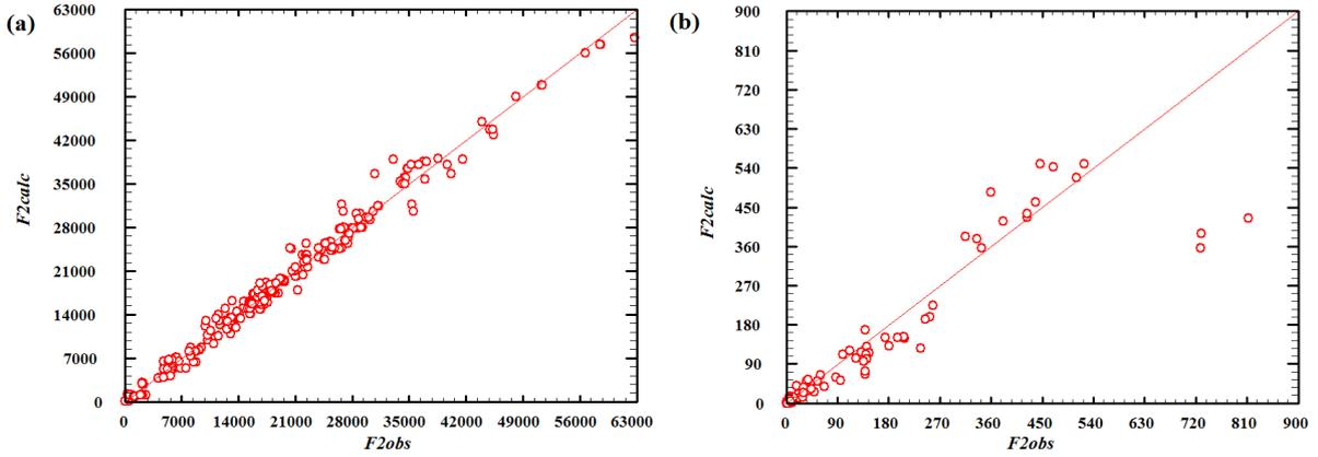
Figure 2: Comparison of the calculated and observed structure factors for (a) the high temperature (300 K) structure refinement and (b) the low temperature incommensurate component refinement.
