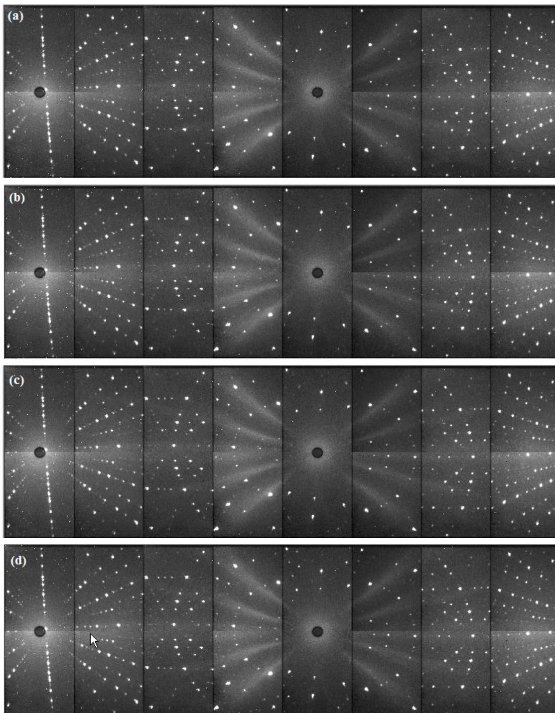
Figure 3: Neutron Laue photographs taken using CYCLOPS. The photos were taken at (a)  $T = 20$  K, (b)  $T = 13$  K, (c)  $T = 6$  K and (d)  $T = 1.8$  K.
