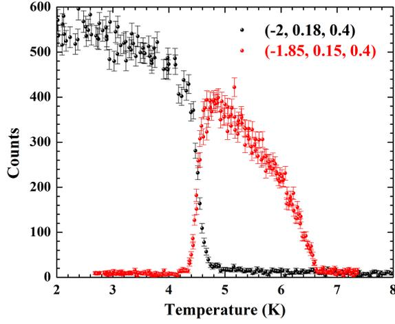
Figure 1: Temperature dependence of the intensity of the two incommensurate peaks in  $\text{NdB}_4$ . Characterisation has shown the purely incommensurate phase occurs between  $T_{N1} = 7.1$  and  $T_{N2} = 4.6$ , while the mixed commensurate and incommensurate phase occurs below  $T_{N2}$ , consistent with our results.
