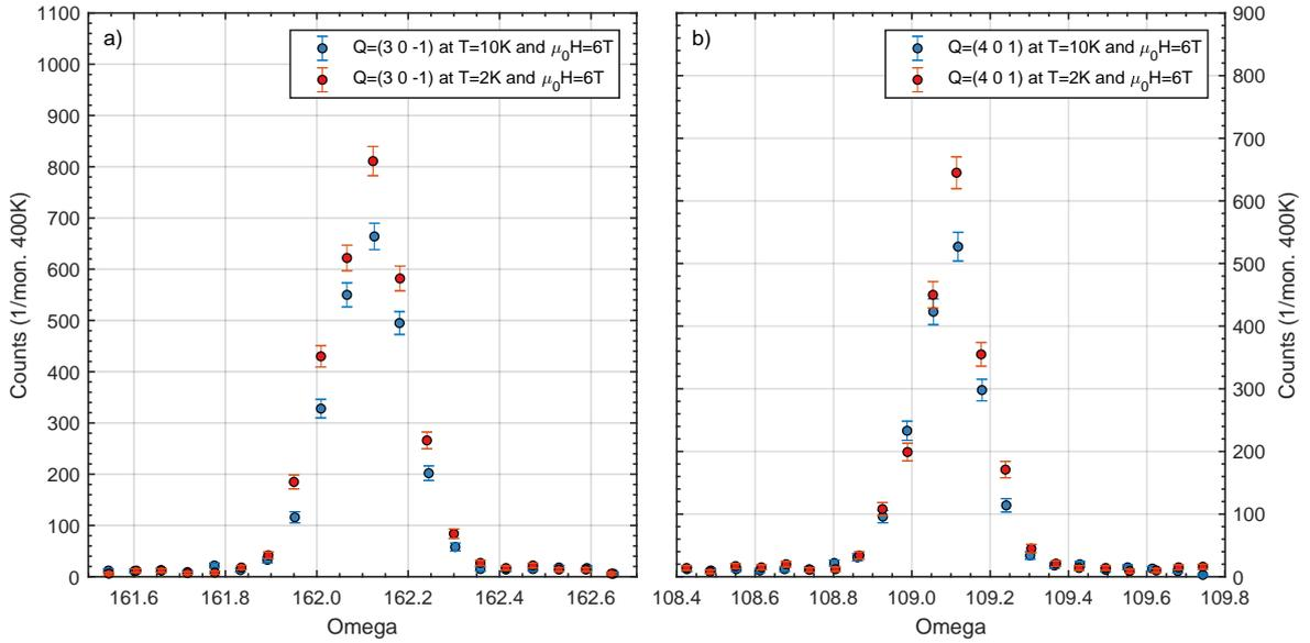
**Figure 1.2: Measurements with an analyzer and a single  $^3\text{He}$  detector**
