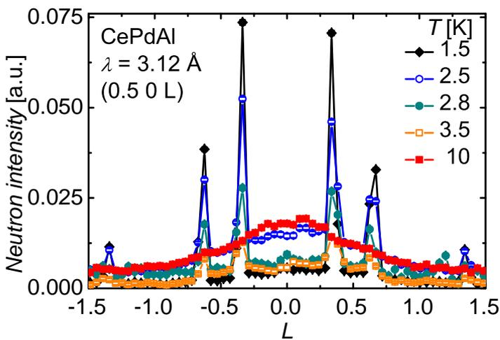
Fig. 1: Scans along  $(0.5 \ 0 \ L)$  in CePdAl measured at different temperatures for neutron polarization along  $z$  and spin-flip scattering.
