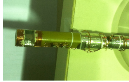
FIG. 1: The coils provided an AC field perpendicular to the applied field. The \text{MgB}_2 sample was located between the two coils
