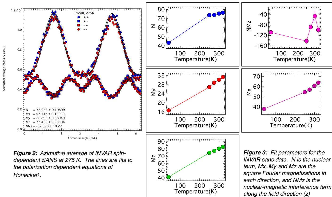
**Figure 2:** Azimuthal average of INVAR spin-dependent SANS at 275 K. The lines are fits to the polarization dependent equations of Honecker<sup>1</sup>.
