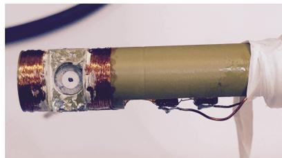
FIG. 2: The MgB<sub>2</sub> crystal mounted on a sapphire disk, in between an AC magnetic field coil.
