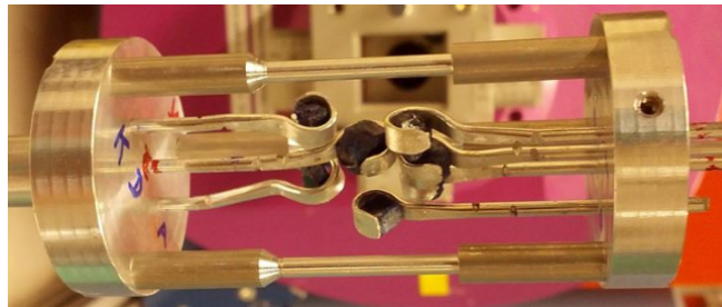
Figure 2: Photo of the co-aligned samples on the aluminum holder with a total mass of 2182 mg.
