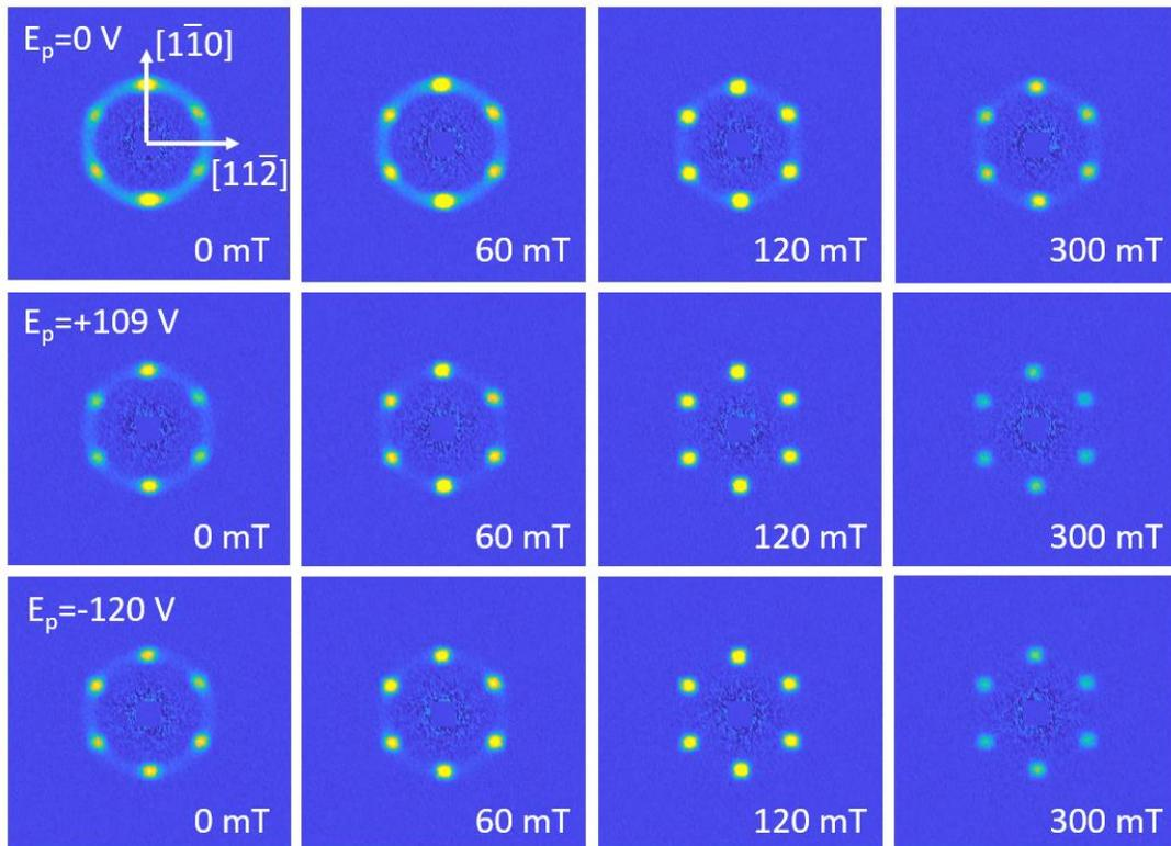
**Figure 1** Magnetic field dependence of the SANS patterns measured for  $\mathbf{k}_i \parallel \mathbf{H} \parallel [111]$  at 12 K. In each row the poling electric field  $E_p$  is the same.
