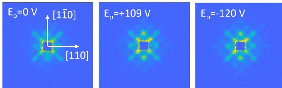
**Figure 2** SANS patterns measured for  $k_i || H || [111]$  at 20 K in the paramagnetic phase after poling the sample with different electric fields.
