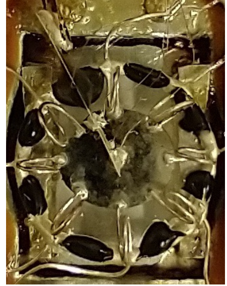
Fig. 1 Corbino sample used in the SANS experiment. The MnSi crystal is resting on a sapphire disk. A HTS is soldered to the center and eight silver wires are attached to the perimeter to produce a radial electric current.
