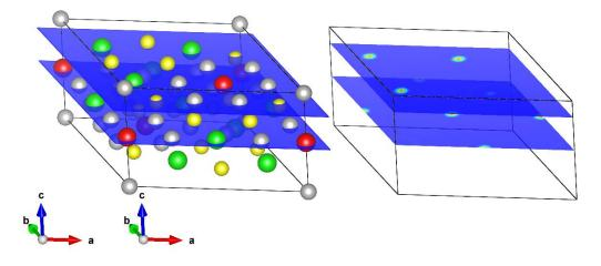
Figure 1 Spin density map as a result of the MAXENT method. Two cuts in the right panel clearly shows large positive spin density on the one set of U sites (marked green in the structural representation in the left panel) and almost zero density on the remaining fourth (red) U ion.
