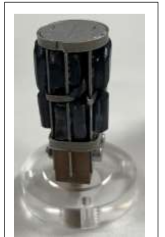
Fig. 1 ~16 g of co-aligned single crystals of \text{Sr}_2\text{RuO}_4 .
