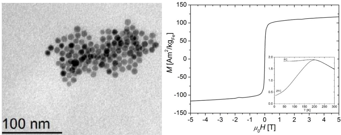
Figure 1—left: TEM image of S2. right: Isothermal magnetization measurement of S2 at  $T = 300$  K (inset: Zero field cooled (ZFC)-Field cooled (FC)-measurement).
