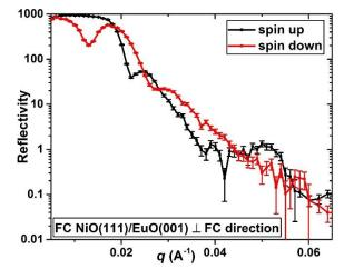
The SF channels show that there is no magnetization induced in the NiO(111)/EuO(001) in the direction perpendicular to the magnetic field applied during the experiment.
