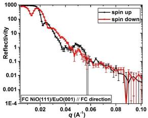
• An induced magnetic moment of 0.89  $\mu_B$ / molecule in the NiO layer 1.3 nm from the interface is deduced from the NSF channels when the sample is aligned perpendicular to FC direction.
