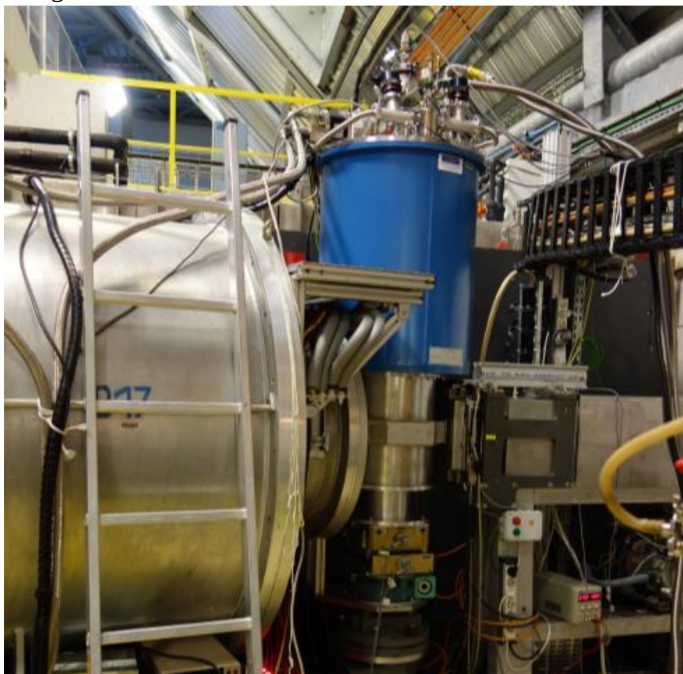
Figure 1 View of the D17 polarized neutron reflectometer equipped with the 7T vertical field cryomagnet.
