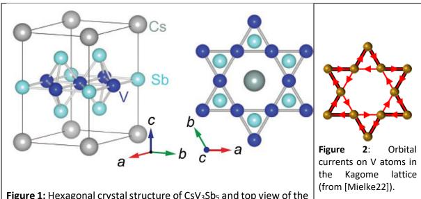
Figure 1: Hexagonal crystal structure of CsV<sub>3</sub>Sb<sub>5</sub> and top view of the Kagome lattice where V atoms are in dark blue.
