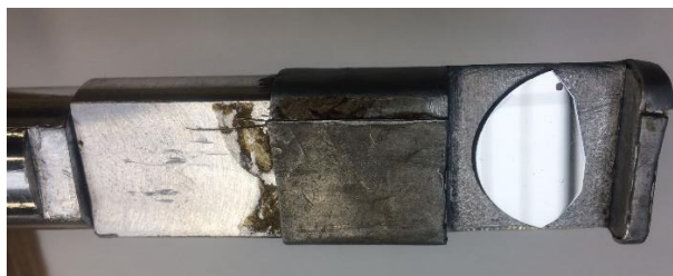
Figure 1: Photograph of the polished MnSi single crystal mounted prior to PNR measurements. The optical reflection of linear lines from the sample surface indicates the surface of the sample has a low roughness required for reflectometry measurements.
