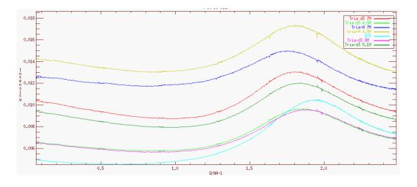
This is a preliminary result: our goal is to measure, in both D16 and D4 instrument, the solvation structure and the nature of the intermolecular interactions of aqueous triazole solutions. The unique resolution and Q-range characteristics of D16 will allow us to study the intermolecular bonding, while D4 yields the necessary information of the interatomic arrangement.
