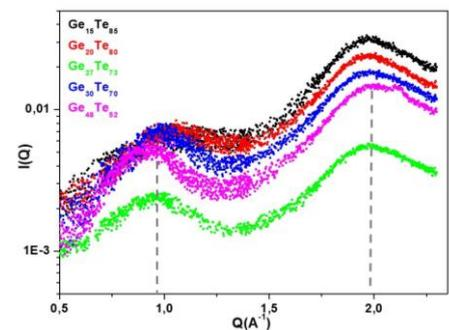
**Figure 3:** Normalised SANS scattering intensity  $I(Q)$  for  $\text{Ge}_x\text{Te}_{100-x}$  glasses in the high- $Q$  range.
