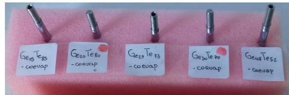
**Figure 1:**  $\text{Ge}_x\text{Te}_{100-x}$  samples placed in non-sealed cylindrical vanadium containers.
