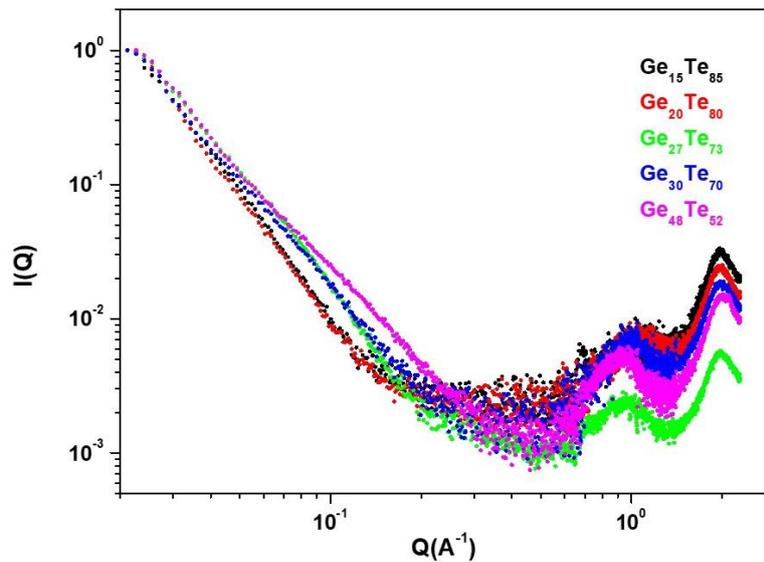
**Figure 2:** Normalised SANS scattering intensity  $I(Q)$  for  $\text{Ge}_x\text{Te}_{100-x}$  glasses elaborated by co-thermal evaporation technique.
