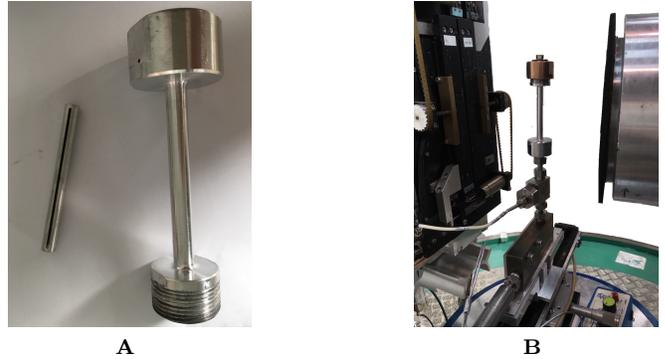
FIGURE 1. (A) High pressure cell and flat thin insert used for the experiment. (B) High pressure cell connected to a fluid separator, water pressure is directly measured at the base of cell.
