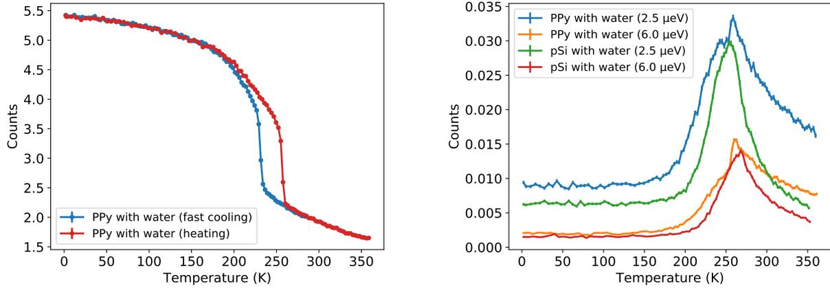
**Figure 1:** (left) Elastic fixed window scans for wet polypyrrole, (right) inelastic fixed window scans with a fixed energy transfer of  $\pm 2.5 \mu\text{eV}$  and  $\pm 6.0 \mu\text{eV}$  for wet polypyrrole and water in porous silicon. All datasets shown in the graphs are averaged over all wave vector transfers  $Q$ .
