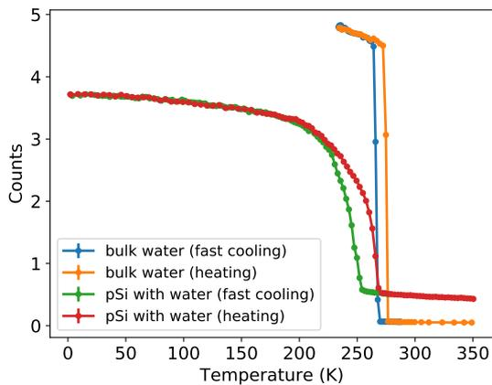
**Figure 2:** Elastic fixed window scan for water in porous silicon nanopores (averaged over all  $Q$ ).
