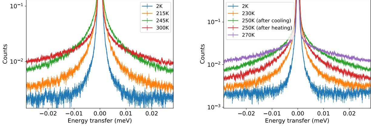
**Figure 3:** QENS spectra (*left*) of wet polypyrrole at different temperatures and (*right*) of water confined in porous silicon membranes (*Q*-averaged spectra).
