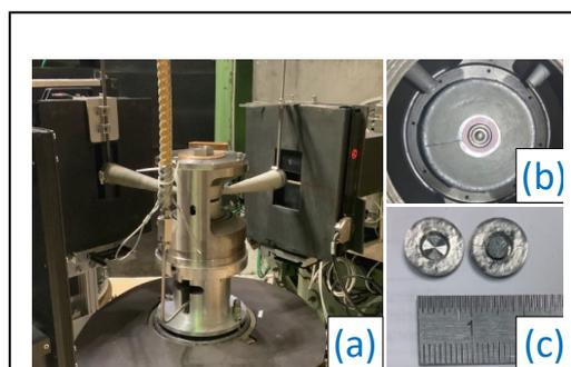
**Fig. 1. Inelastic Neutron Scattering experiment setup at IN8, ILL. a,** geometry with two cones (incident beam; scattered beam) and two anvils (on/below the sample shell), high pressure oil pumped through steel pipe. **b,** folded encapsulating gaskets, within which is full of alcohol liquid. **c,** PbTe sample and gasket demission.
