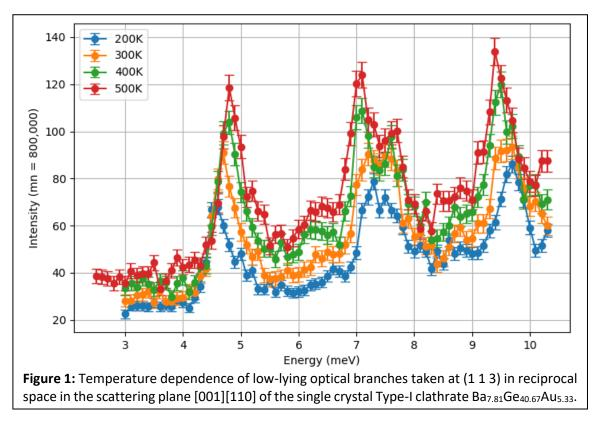
As expected, the lowest branch at 4.9 meV shifts higher in energy with temperature while the next two branches shift down in energy with temperature. Further analysis will have to be done in order to understand why the second branch appears to split into two modes at higher temperature. This is most likely due to the fact that optical phonon branches are each a series of modes, and therefore it is possible that not all modes in a given branch have the same temperature dependence.
