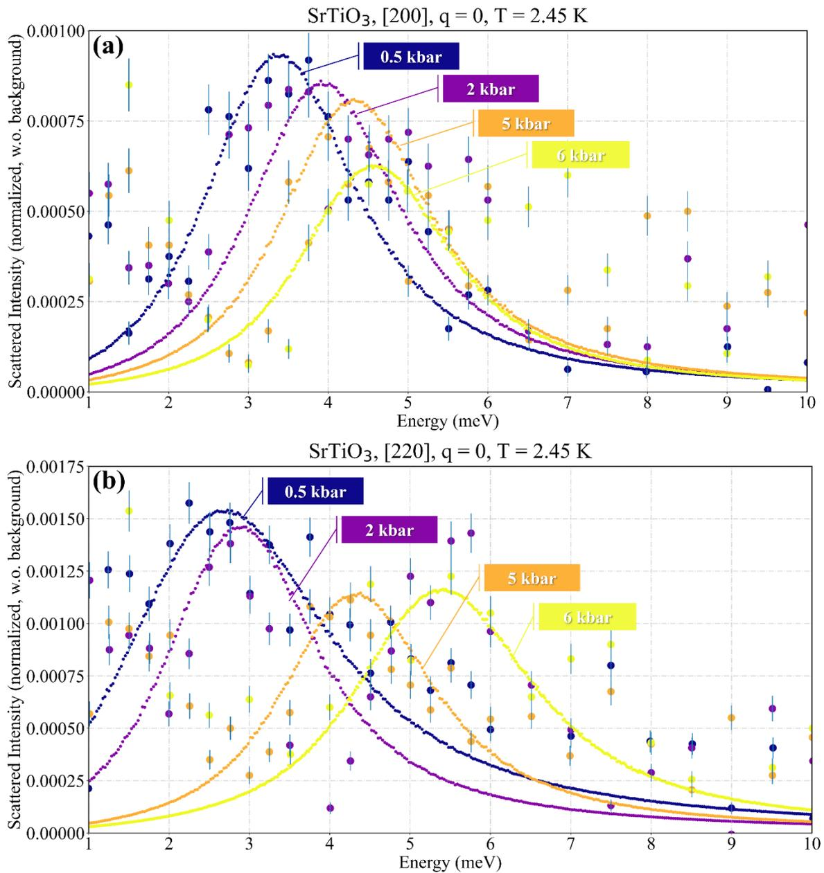
**Fig.2** The Brillouin zone centre ( $q = 0$ ) energy scans under pressure from 0.5 up to 6 kbar at  $\sim 2.45$  K around the (200) and (220) Bragg peaks. The background contribution from the pressure cell has been subtracted. And the intensity from the sample itself has been fitted with *Takin2.0* to deconvolute the triple-axis resolution on IN8, shown in the dense dotted lines.
