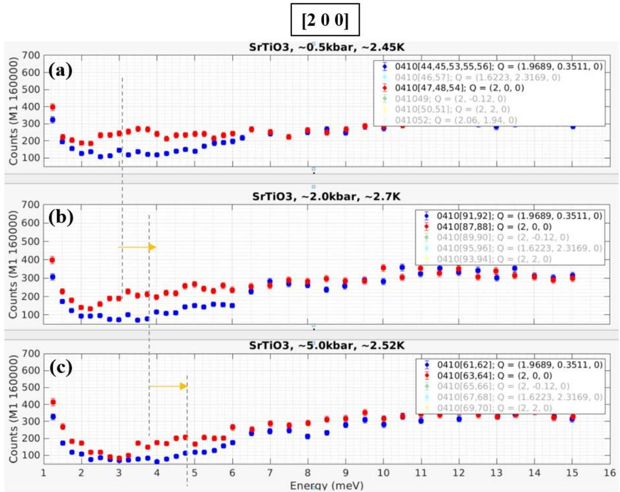
**Fig.1** The Brillouin zone centre ( $q = 0$ ) energy scans under pressure at 0.5 kbar (a), 2.0 kbar (b) and 5.0 kbar (c) at (200) Bragg peaks. The red dots represent the STO sample together with the background from the gas gate pressure cell. The blue ones represent the corresponding background scans.
