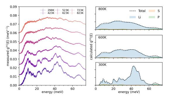
The signal is visibly dominated by the Li displacements of interest. Moving from the room temperature  $\gamma$ -phase of interest to the superionic  $\beta$ - and  $\alpha$ -phases the GDOS visibly broadens and the phonon band centers shift to much lower energies (soften). This is in accord with Raman- and impedance-spectroscopy results and will be published soon<sup>TM</sup>.
