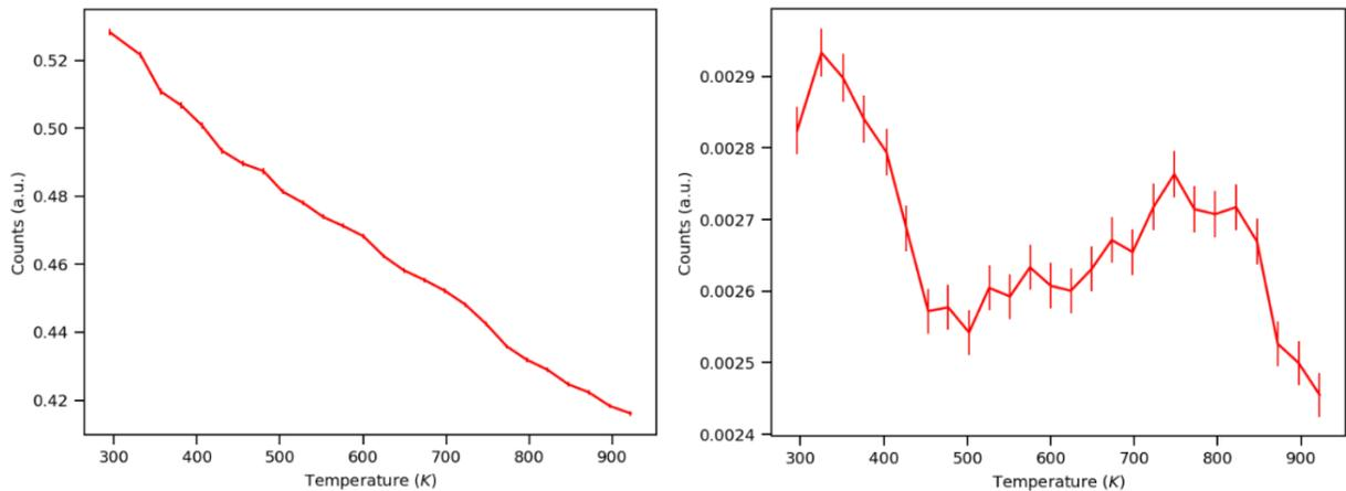
Figure 1. Elastic fixed window scan (left) and inelastic fixed window scan (right) of  $\text{La}_{1.54}\text{Sr}_{0.46}\text{Ga}_3\text{O}_{7.27}$  collected on IN16B on heating.
