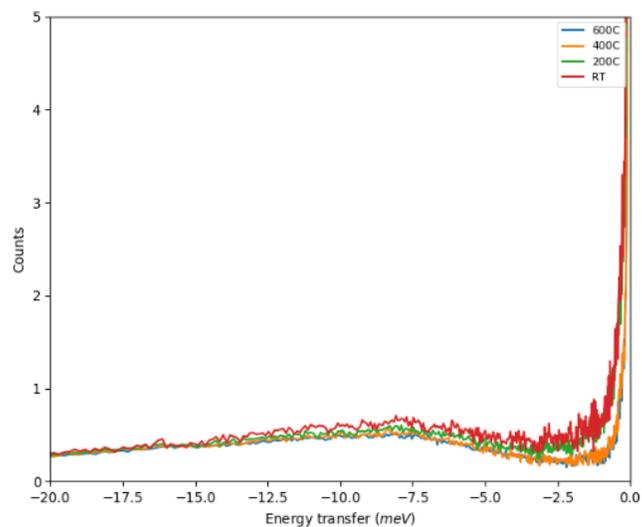
Figure 2. The Q-integrated scattering function corrected for the Bose population factor against energy transfer at several temperatures for  $\text{La}_{1.54}\text{Sr}_{0.46}\text{Ga}_3\text{O}_{7.27}$  measured on IN6.
