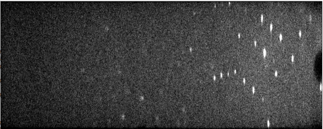
Diffraction observed from triclinic HEWL at 100 K. From partial data collected at D19, June 2016.
