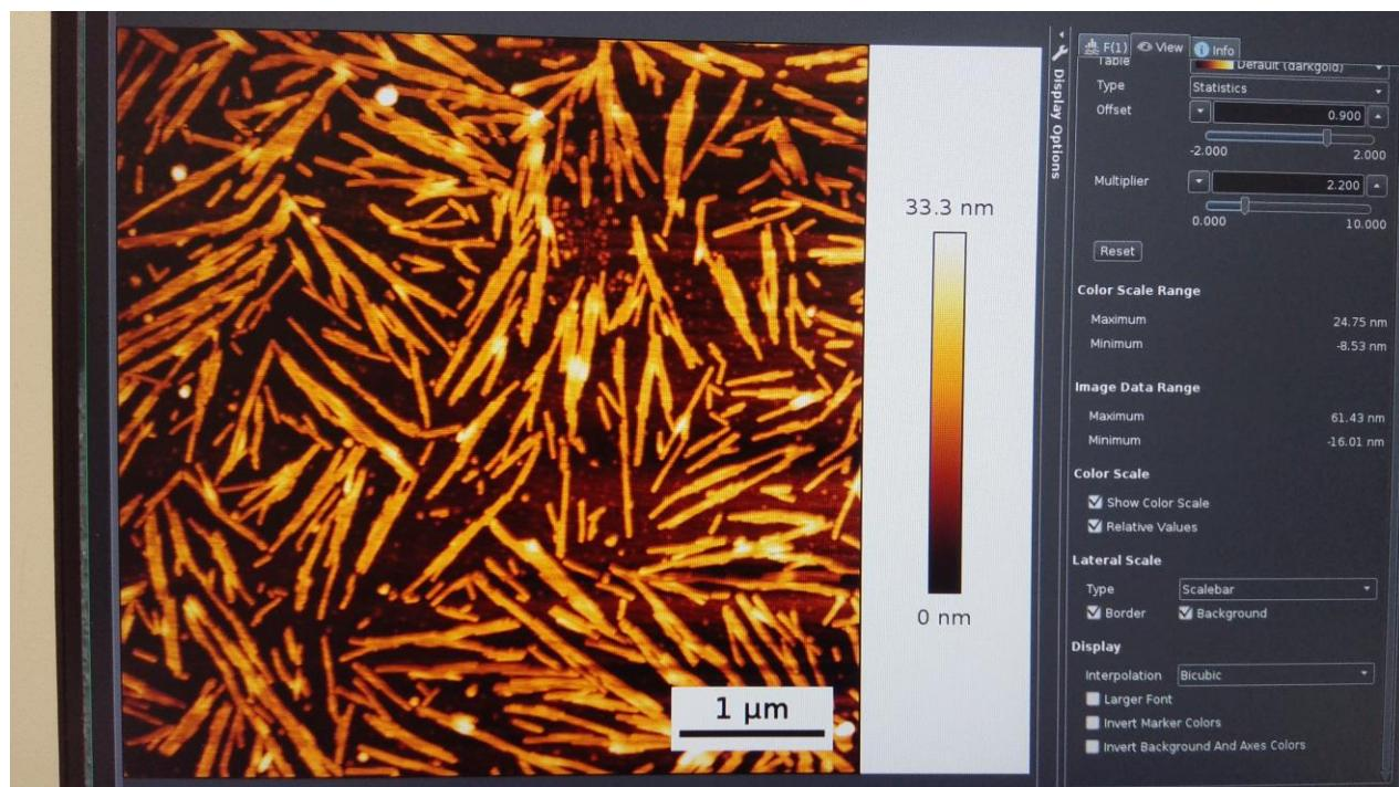
*AFM scan (noncontact mode) of a large area of the Si wafer (dark brown), covered by well-adsorbed viruses (light brown). The scan was recorded after many hours of exposure to the neutron beam.*
