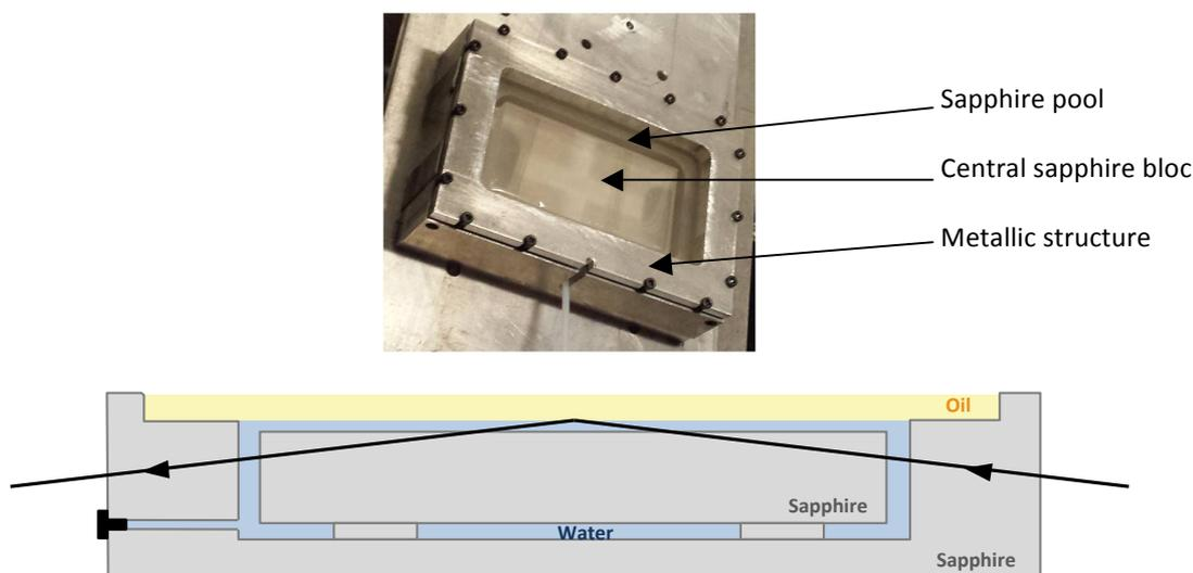
**FIGURE 1: Picture of the cell in the metallic structure and sectional view of the filled cell.**
