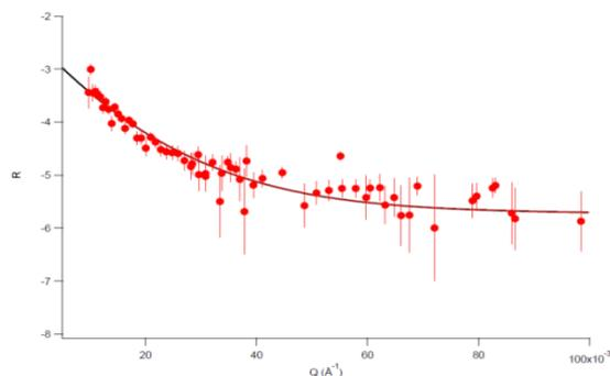
**FIGURE 6: Reflectivity curve for a water/H-isopropyl myristate interface ( $SLD_{\text{isopropylmyristate}} = 0 \text{ \AA}^{-2}$ )**
