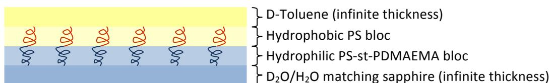
**FIGURE 4: The 4-layer configuration used to fit the data**
