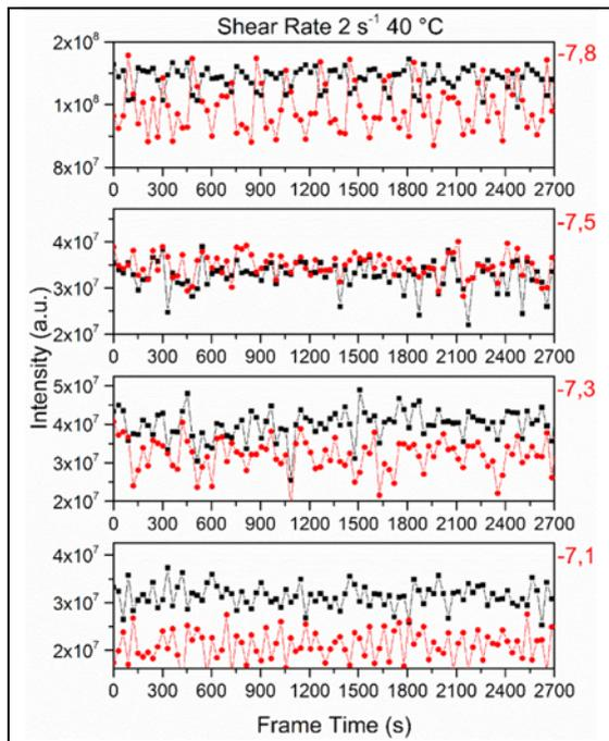
Figure 2: SANS intensity at the two Bragg peaks at 110° and 290° (averaging 20°) as a function of time (red and black respectively). The Figure reports the intensity behaviours at all 4 gap positions.
