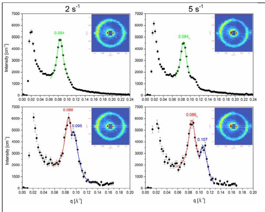
Figure 3: Scattering profiles of selected 2D SANS patterns at 2  $s^{-1}$  (left) and 5  $s^{-1}$  (right) at 45 °C. The figures on top are radial average of the overall 2D pattern, while the profiles in the bottom are average of the selected zone (white rectangular). Patterns collected at the outer wall position (-7.8).
