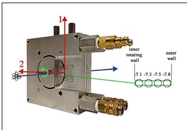
Figure 1: 1-2 shear cell allows scattering in the 1-2 plane. The 1-, 2-, and 3- directions are defined as the velocity, velocity gradient and vorticity directions, respectively. The position in the couette gap were defined by using the table with x,y,z,w positioning plus (q)-goniometer. Position -7.1 along x correspond to the point closer to the inner wall, while -7.8 to the outer wall.
