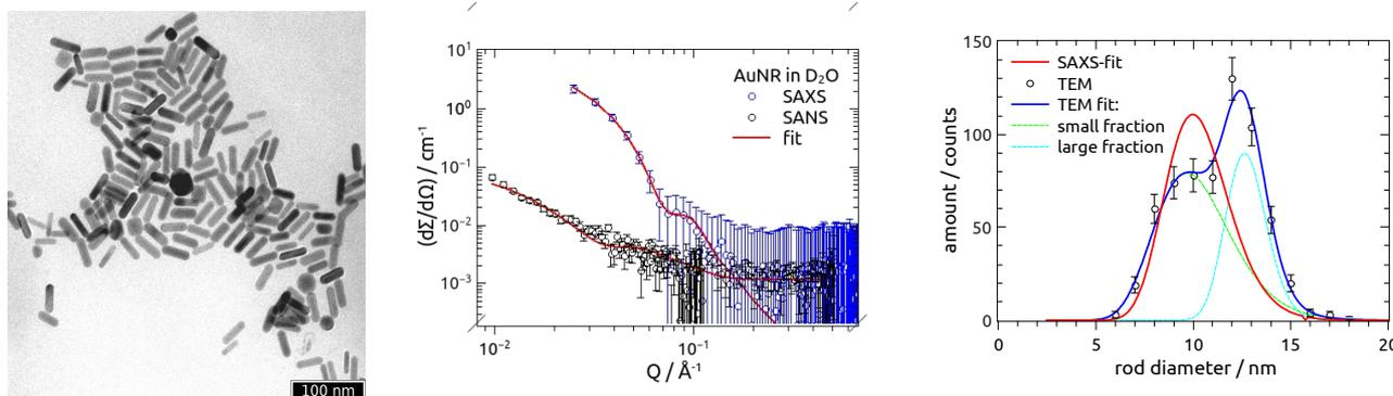
**Fig.1:** TEM image (left) of the sample used for further SAS analysis showing gold nanorods and a small amount of non rod-like particles. Fitting the SAS data (of SANS @ D11 and SAXS @ our laboratory instrument) simultaneously is very sensitive to the rod diameter distribution and can be compared directly to the values gathered from quantitative TEM analysis (right).
