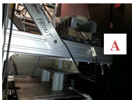
Figure 1. (A) Picture of Experimental setup for lead shielding around the gamma detector. (B) Gamma intensity as a function of wavelength recorded during previous beamtime at ILL. (C) Gamma intensity as a function of wavelength during the last beamtime on FIGARO. Thanks to the lead shielding we can observe that the signal to noise ratio in the gadolinium emission line increases considerably.
