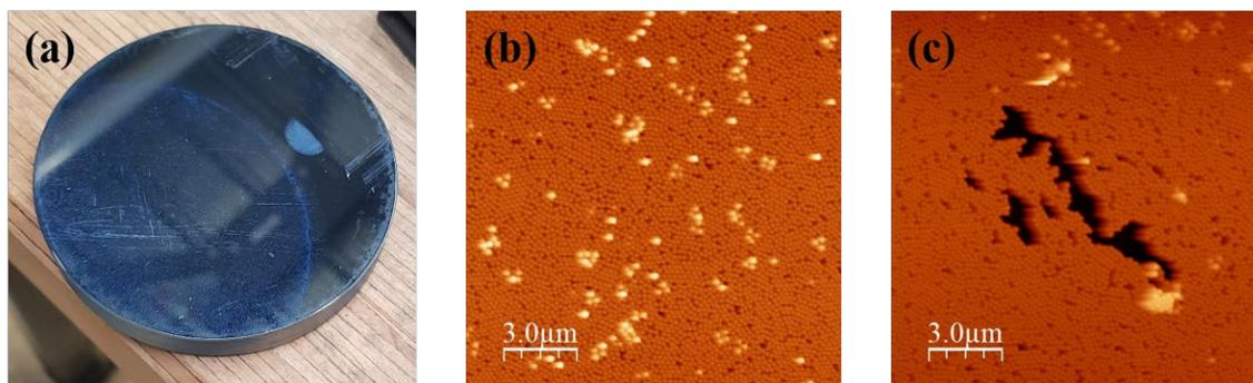
**Figure 3.** **a)** Silicon block with the silica nanoparticles on top, after being sheared. The brighter blue region corresponds to that in contact with Melinex during the whole experiment. The darker blue region corresponds to a sheared region that moved away from the area in contact with the Melinex during the experiment. **b)** and **c)** AFM images of the bright and dark blue region of the block in (a).
