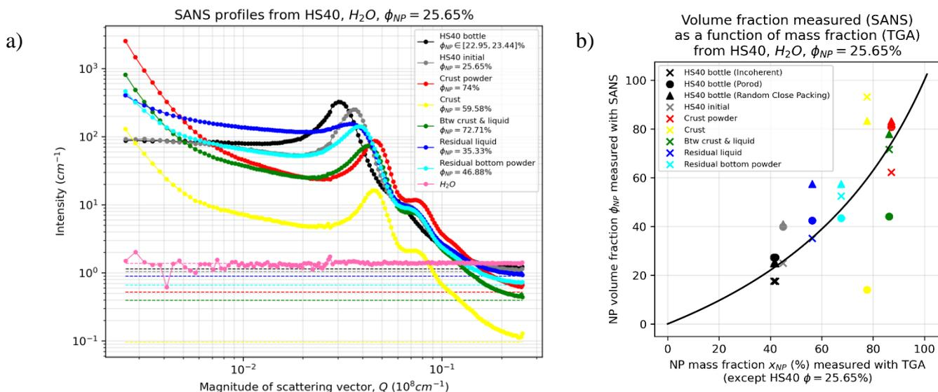
Fig.4: SANS results for HS40. a) Spectra. b) various determinations of the NP volume fraction.
