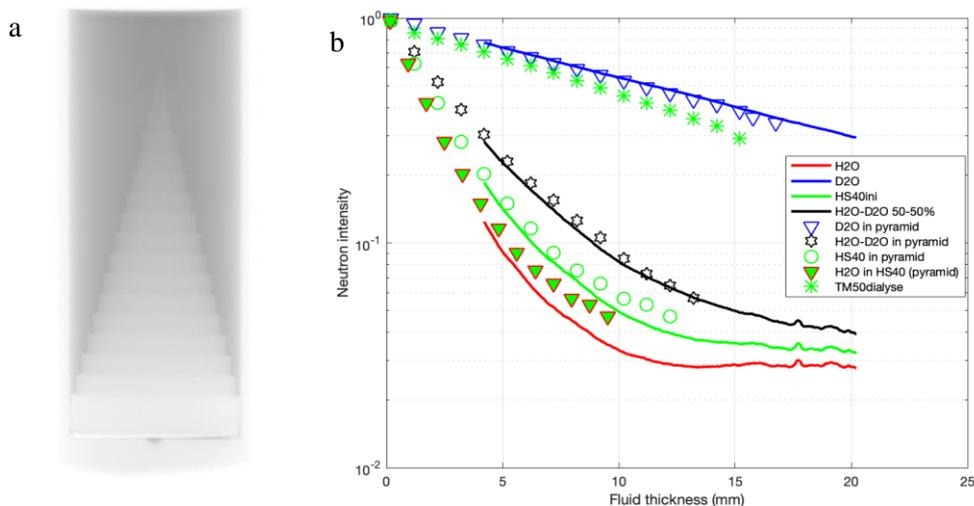
Fig.3: Calibration of the neutron transmission intensity as a function of the fluid thickness. a) snapshot of the calibration pyramid in D<sub>2</sub>O (inner diameter=16.76mm). b) calibration measurements with the triangular cell at 7cm from the detector, i.e. at
