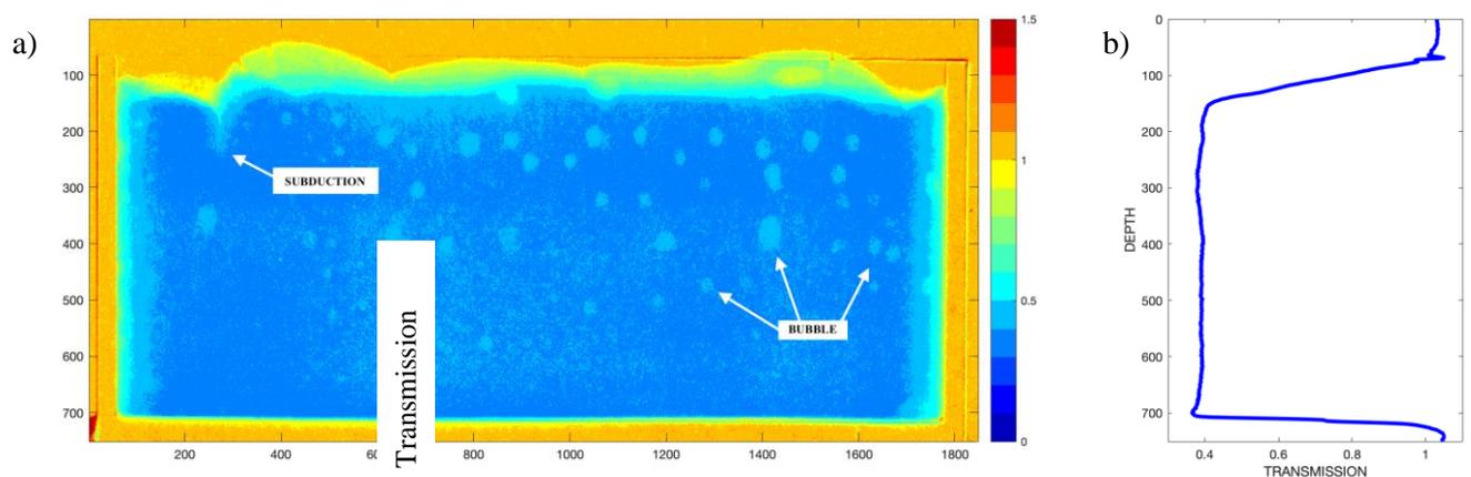
*Fig.2: Neutron transmission for the experiment with TM50 dialysed in D<sub>2</sub>O. a) snapshot at time  $t=360$  min. The top interface is showing folds and a subduction on the left. Air bubbles caused by the heating are also visible. b) Depth profile of the transmission average along the cell.*
