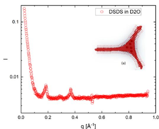
Figure 2 Scattered intensity as a function of  $q$ -vector for foam stabilised with DSDS precipitated in the presence of KCl.
