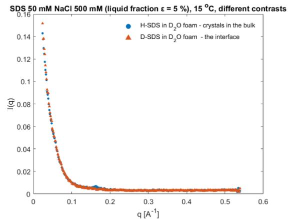
Figure 5 Scattered intensity as a function of q-vector for a foam stabilised with deuterated SDS precipitated in the presence of NaCl.
