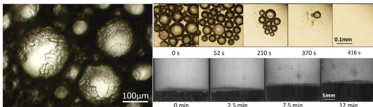
Figure 1 Surfactant crystals on bubble surfaces visualised under the microscope (left). Destabilisation of bubbles and foam through heating (right).
