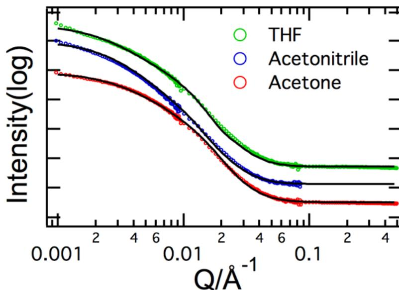
Figure 1. SANS profiles for PLGA-PEG nanoparticles prepared with different solvents via a nanoprecipitation method measured in D<sub>2</sub>O. Solid lines are the best fit to the data.
