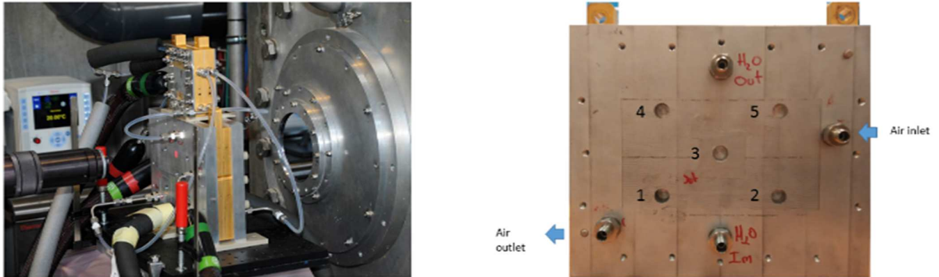
Figure 1: Experimental setup for the reference measurements, with the small surface cell on top of the (left), and a picture of the cell with the positions annotated (right).
